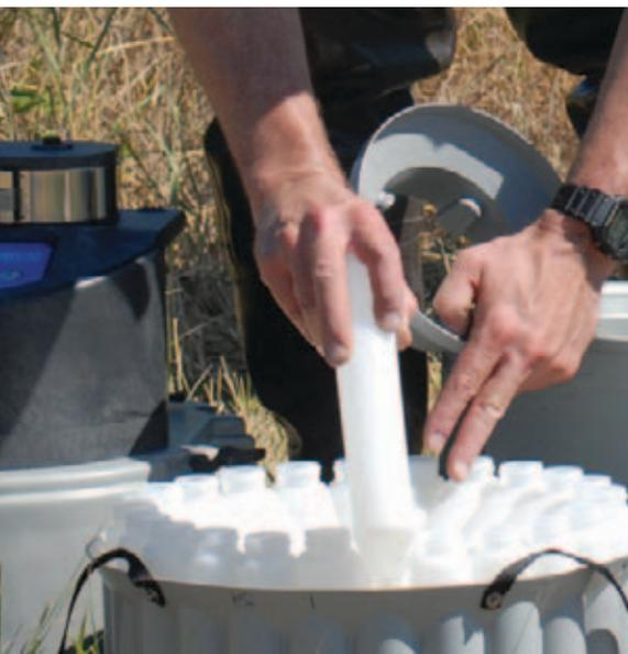
**Bottles, suction lines, and strainers contact the sample liquid. Always select wetted materials that are compatible with the sample analysis.**
